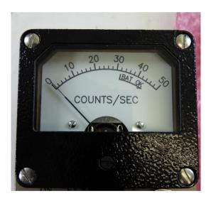
It should be noted that the STS electronics draw a significant current whilst sensing and so although the battery icon may suggest the batteries are ok please change them before any other action is taken. The Ludlum 3 requires 2 D cell batteries.
