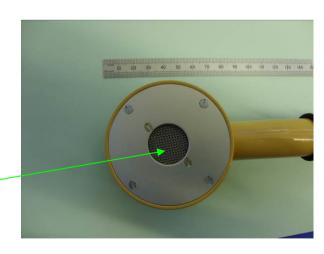
Looking at the perforated face plate of the probe remove the 4 outer screws through the cover and set aside.
