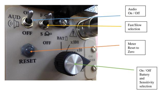
When using it must be noted that the probe must be connected to the instrument and the connectors done up before the instrument is turned on, failure to do this may cause the initiation of the system to fail and result in no detection of the stimulant.
