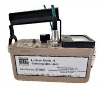
The STS 808 Ludlum 3 simulator retains the same controls and options as the real instrument.
