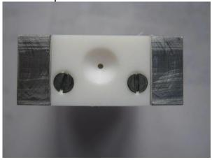
Reassemble the detector block by inserting the spring with the gauze end against the top
