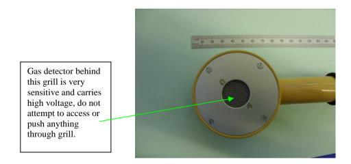
Looking at the perforated face plate of the probe remove the 4 outer screws through the cover and set aside.
