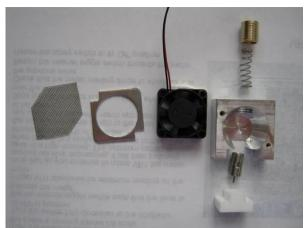
Once removed carefully undo the two screws through the detector plate. Before complete removal note the correct assembly of the components held by the screws. Remove the screws and carefully set aside the wire gauze and spacer, move the fan from the detector block to expose the brass tube mounted in the side of the detector.
