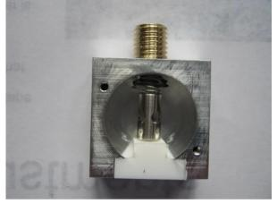
Unscrew the two screws through the white plastic block and carefully ease the detector out and replace with a new detector.
