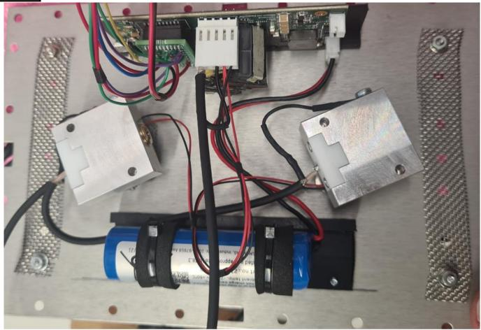
The 2 pozi screws either side of the circular hole can then be removed to release the detector block and enable the detector to be changed.
