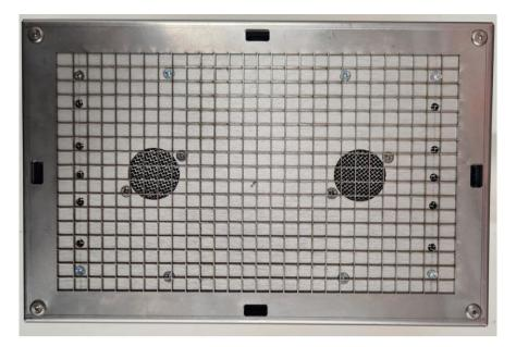
Lift off the cover plate to reveal the plate below. – remove the 20 torque screws holding the plate to the body.
