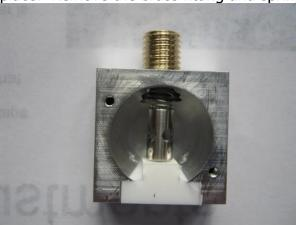
Unscrew the two screws through the white plastic block and carefully ease the detector out and replace with a new detector.
