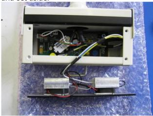
Carefully lift the detector plate from the probe body and disconnect the 5 way connector mounted on the circuit board. Care must be taken not to remove this by pulling on the wires which may cause damage.
