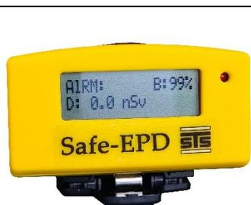
The STS Safe-EPD simulator is a simulated generic Electronic Personal Dosimeter designed to aid the tuition of workers in the nuclear industry in safe practices and in understanding the accumulation of dose over time but without exposure to radiation.
