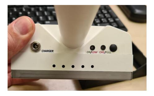
If the Led is lit red then the unit should be put on charge. Use only the supplied charger to charge the unit (6V @2A max) – the unit will take 6-8hrs to fully charge.
