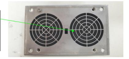
Remove the 8 screws through the face plate.
