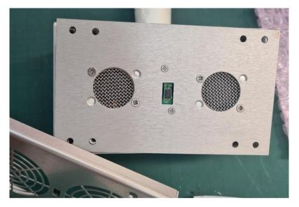
The 2 screws either side of the circular hole can then be removed to release the detector block and enable the detector to be changed.
