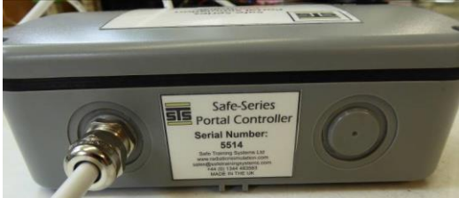
Cable to Portal Detector
