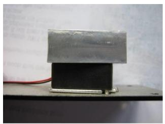
Align the face plate with the holes in the probe body and replace the 8 screws.
