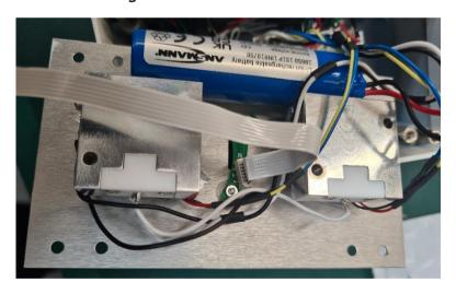
Before complete removal note the correct assembly of the components held by the screws. Remove the screws and carefully set aside the wire gauze and spacer, move the fan from the detector block to expose the brass tube mounted in the side of the detector.
