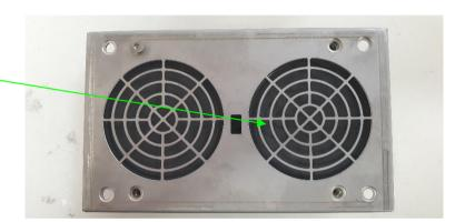
Remove the 8 screws through the face plate.
