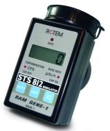
The STS 812 Ram Gene simulator provides a contamination only simulation. To monitor remove the cap, the led will light to show CPS has been selected. The subject may now be monitored by moving the instrument slowly over the clothing keeping the unit within 1 cm of the surface.
