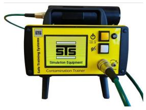
All STS contamination monitors are based on real instrument with additional STS electronics built into them or are wholly manufactured by STS such as the Contamination Trainer and CMS. User controls, screens and instrument functions are either retained or duplicated to provide the most realistic training environment.
