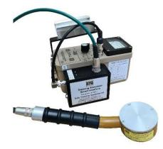
Alternatively, where users wish to use small frisker style probes such as an HP260 you can use the Training Simulator Smart interface (TSSI) which connects directly to a real meter and the Standard STS probe connecting to the interface.
